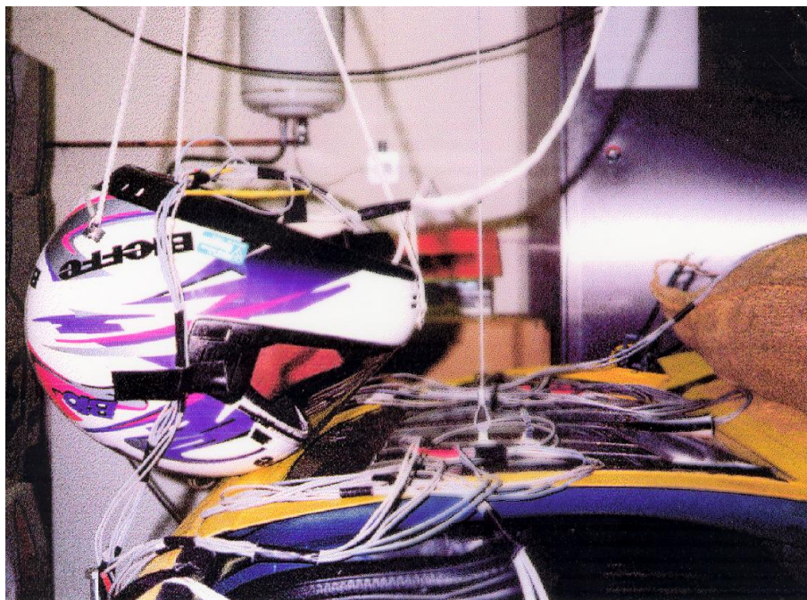
Figure 5.1: Example of a TRL accident reconstruction test
